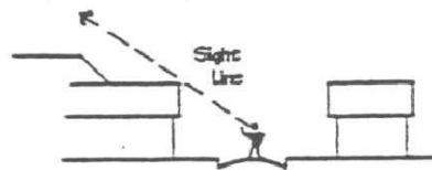
STEPPED BACK NEW CONSTRUCTION
