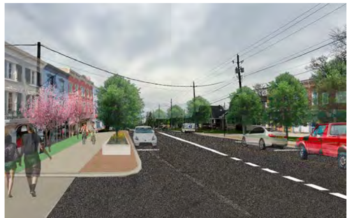
CONCEPTUAL AFTER - Adding clear sidewalks separated from the roadway with landscaped bump outs and on-street parking
