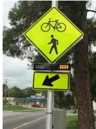
Ground Mounted RRFB
