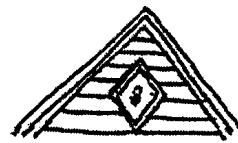
APPROPRIATE Attic vent retained
